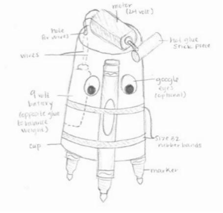
that is spinning around the outside of the motor. Since the motor is spinning really fast, it's really throwing the weight around and making the whole Draw Bot wiggle. As the Draw Bot wiggles around the paper, the markers leave a really cool design!
