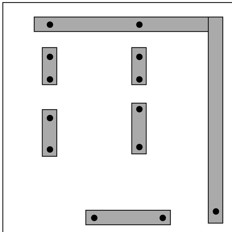
2. Cut strips of tin foil tape to the right length and press them down firmly on the circuit board pattern.
