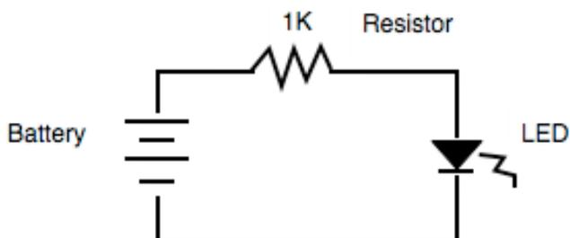
*Resistors are measured in Ohms. What happens when we put in a 1 K Ohm resistor, or a resistor that measures 1000 Ohms of resistance?*
