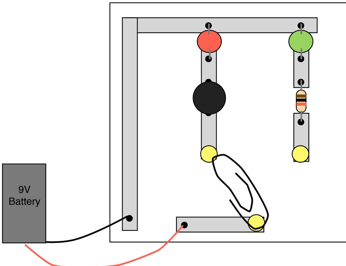
11. Attach the battery and test! What can you use the Tin Foil Circuit Board for? What can a red and green light be used for? True/False, Stop/Go etc.
